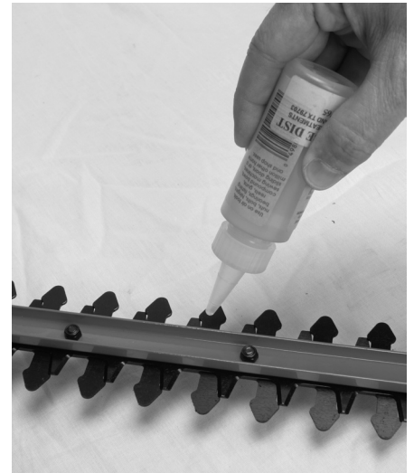
Figure 4-3 : Lubrification des lames
